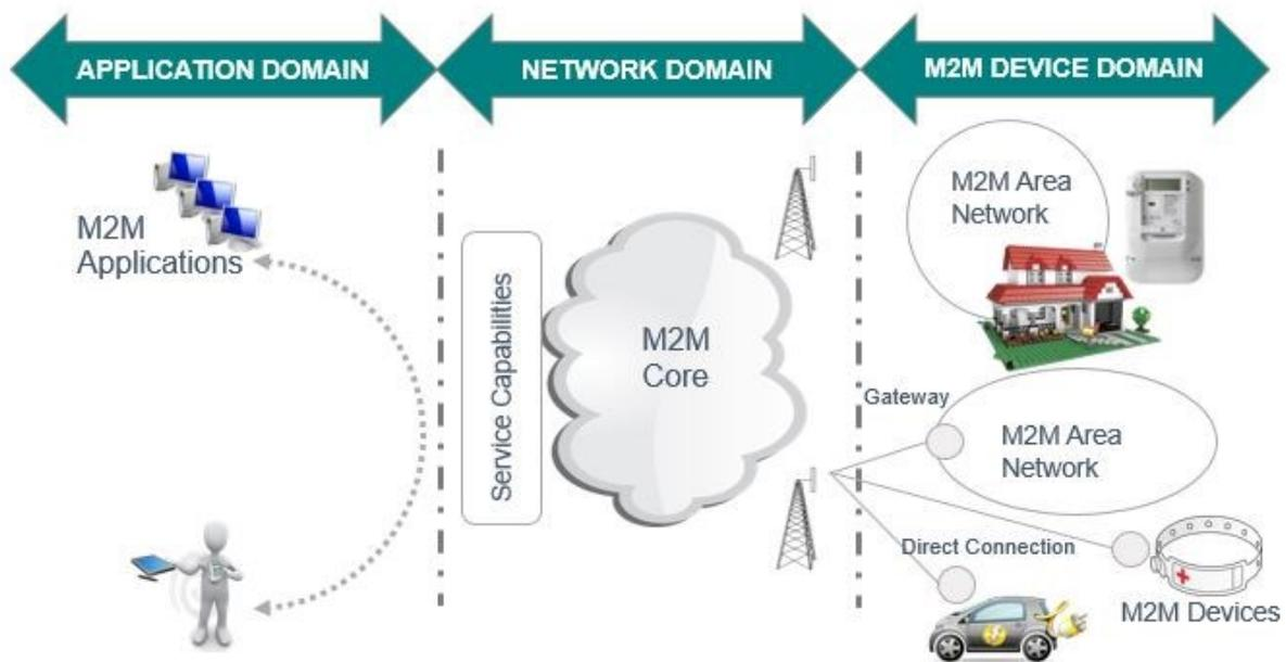
Fig 3: The ETSI M2M Architecture
