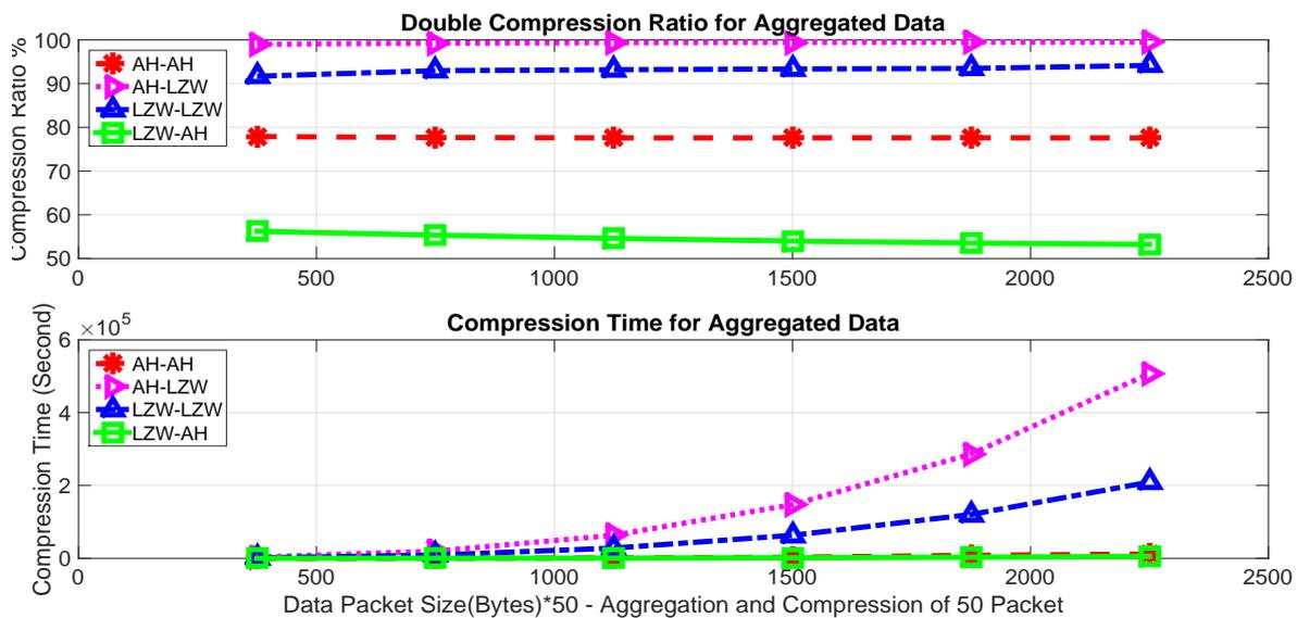
Figure 15: Results for compression ratio (top figure) and compression time (bottom figure) vs packet size for double compression without decompression in aggregator (scenario 3).
