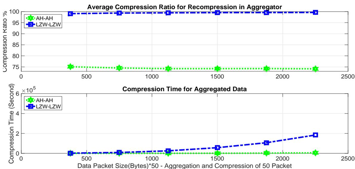
Figure 14: Results for compression ratio (top figure) and compression time (bottom figure) vs packet size for decompression in the aggregator followed by compression of aggregated data (scenario 2).
