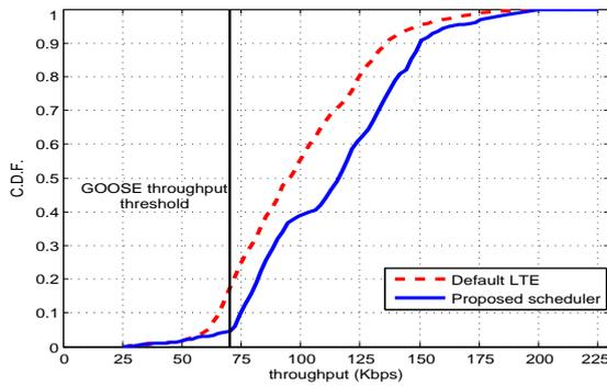
Figure 7: CDF of throughput for GOOSE traffic.
