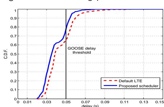
Figure 6: CDF of delay for GOOSE traffic.
