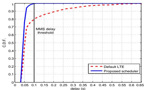
Figure 3: CDF of delay for MMS traffic.
