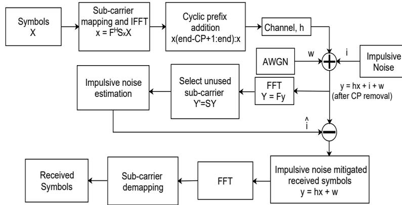
Figure 9: Block diagram of the proposed IN mitigation algorithm.
