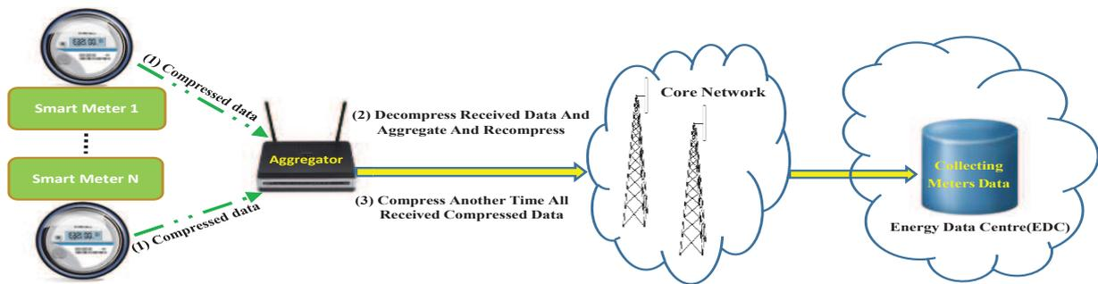
Figure 12: Metering infrastructure and network topology showing the aggregation scenarios 1,2 and 3.
