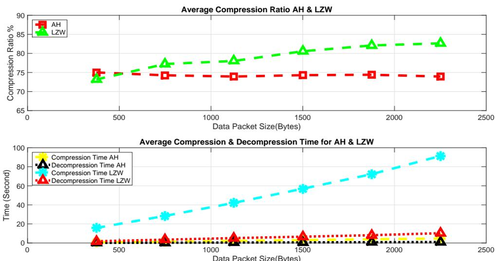
Figure 13: Average compression ratio (top figure) and average compression time (bottom figure) for LZW and AH algorithm applied to meter data in 10 mins intervals (scenario 1).
