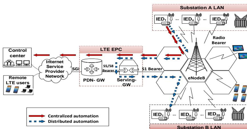
Figure 1: LTE for centralized and distributed substation automation [3].
